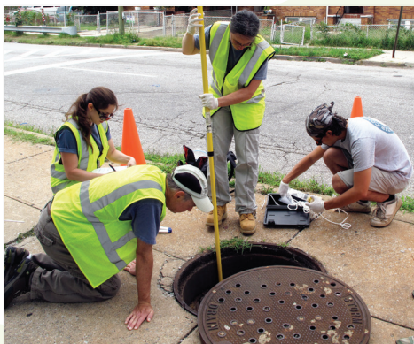
The Center for Watershed Protection works with Blue Water Baltimore and Baltimore City to check storm drains for evidence of sewage discharges. Photo credit: Waterfront Partnership of Baltimore.
